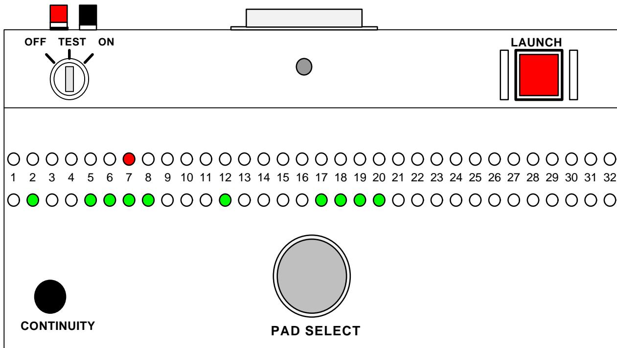
Approximate Layout of the Main Control Console Front Panel.
