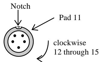
Front view of a typical panel-mount signal connector.
