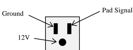
Front view of a typical panel-mount outlet.
